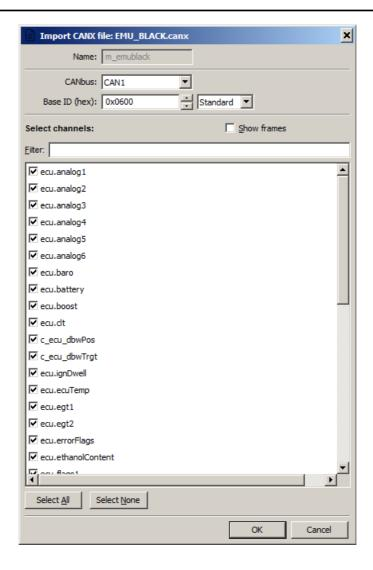
In this menu you should select the CAN BUS network that will be used for communication (CAN1 or CAN2) and which channels you want to read. In most situations all channels should be loaded (Select All). The project tree should look like the following:
